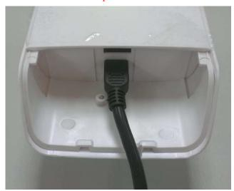
Step3: Install the upper housing Make sure the housing is well installed.
