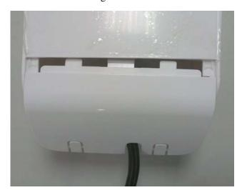
Warning! Do not cover or block the airflow to the adapter. The adapter will reach a high temperature during use.
